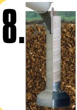
Place rebars (optional). Fill with concrete. \*Note: under dry conditions concrete pour can be delayed up to 48 hours.
