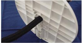
The shield is now on the mooring line and ready to be deployed.
