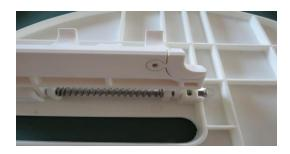
Make sure that the insert is fully seated in the door as shown in this picture. Use the stainless steel screw provided and place it into the retaining hole until it is all the way in. Do not over tighten.
