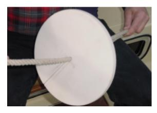
6. The shield is now on the mooring line and ready to be deployed.
