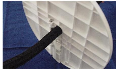
The shield is now on the mooring line and ready to be deployed.
