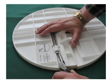
3) You may want to use a glove over the spring at this point. While pulling the bolt out, hold your hand over the spring so that as the bolt is withdrawn the spring does not fly off the door. **Retain the spring**.
