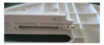
Make sure that the insert is fully seated in the door as shown in this picture. Use the stainless steel screw provided and place it into the retaining hole until it is all the way in. Do not over tighten.
