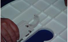
Tighten the two screws equally until they are fully screwed into the door. This will draw the plug-ins even tighter into the door. Do not over tighten.
