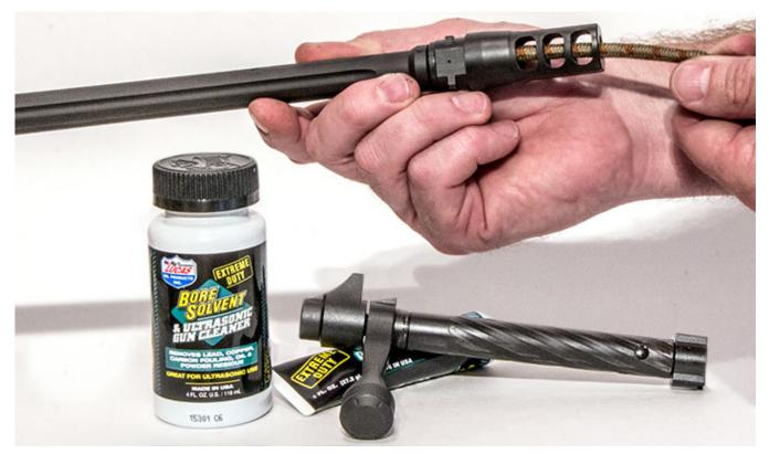
Small parts, like bolts and carriers, can easily fit in ultrasonic cleaners, whereas barrels still need to be cleaned by hand (and from breech to muzzle).
