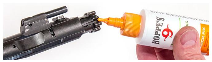
The application of lubrication to a firearm should be done sparingly. More is not necessarily better.
