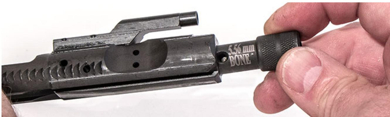
*Specialized components don't necessarily need dedicated gear—like this Otis Bone tool for AR bolt carriers—but having precise means of cleaning and lubricating make the job quicker and much easier.*
