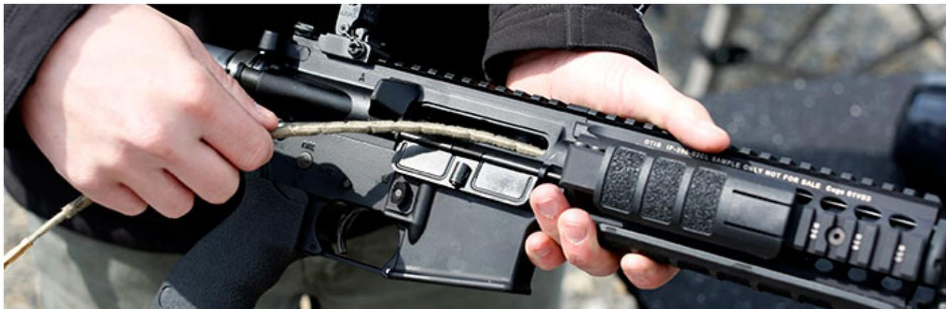
*For quick cleaning in the field, a BoreSnake or Ripcord allows cleaning from the breech without having to completely disassemble your rifle.*
