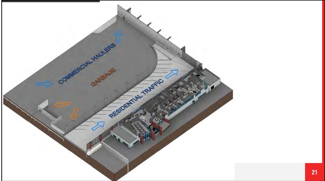
One of the many improvements to the new facility is a more efficient residential experience when they are dropping off trash. Not only will there be additional bays within the Central Transfer building, they will be angled in such a way to allow for easier access. The angle will allow vehicles to back in and out of the spaces quicker, thus decreasing the turnaround time.
