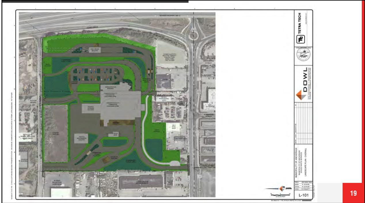
Stormwater runoff from the paved areas of the site will be directed to low lying areas around site to provide treatment before being directed to assist in recharging the on-site wetland located at the northeast corner of the site. An overflow pipe extends from this wetland area to the municipal storm drain system in East 56<sup>th</sup> Avenue to assist in directing stormwater runoff away from the site during larger storm events.
