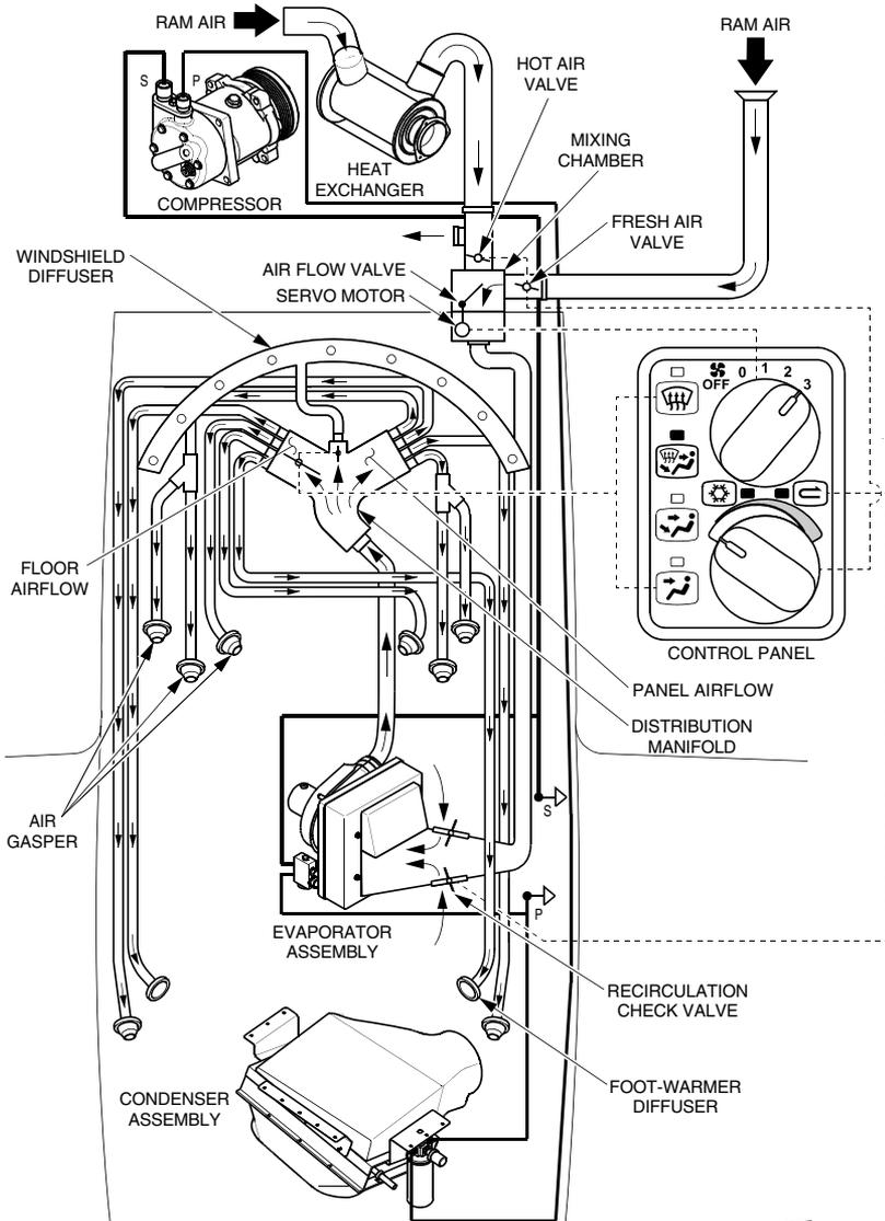
**NOTE:** Illustration depicts maximum cabin cooling airflows and selector settings while on ground or warm outside air temperatures.
