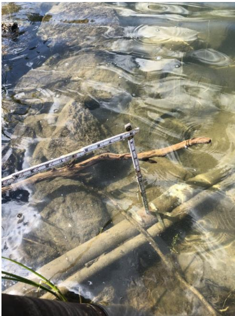
Measuring the water column or gage height.
