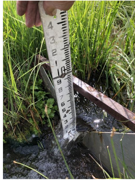
Measuring the flow through a "V-Notch" device.
