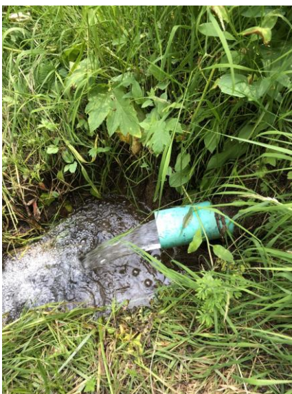
A seep collected through a pvc pipe for ease of measuring.
