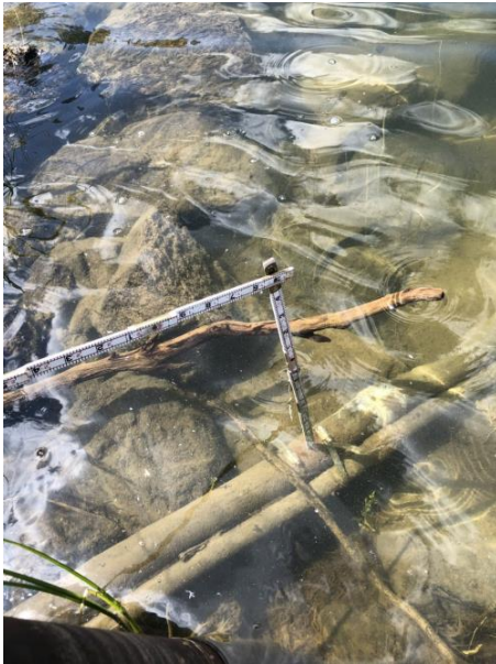
Measuring the water column or gage height.
