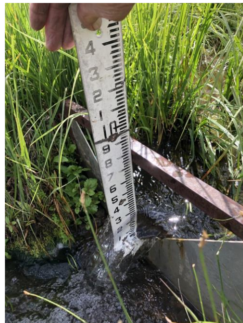
Measuring the flow through a “V-Notch” device.
