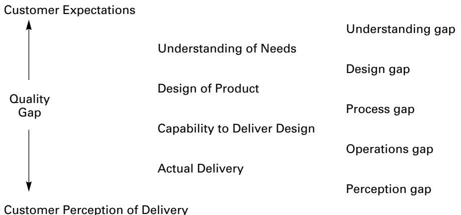
FIGURE 3.1 The quality gap and its constituent gaps. [Inspired by A. Parasuraman, Valarie A. Zeithami, and Leonard L. Berry (1985). “A Conceptual Model for Service Quality and Its Implications for Further Research.” Journal of Marketing , Fall, pp. 41–50.]
