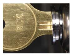
Improper lock core installation is noticable as the lock core will not be flush with the lock core housing.
