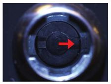
If lock core notch-out is aligned to the right (locked position) or anywhere in between, then the lock core will not install properly.
