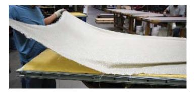
Lay out the new fabric with the correct side up and proper direction (compare with existing panels if unsure). Smooth out any wrinkles that may exist.
