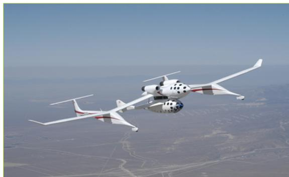
Figure 11.7: *Space Ship One carried aloft by the White Knight carrier aircraft.*
