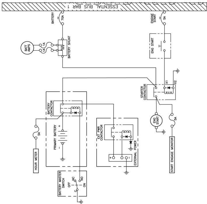
ALTERNATOR AND STARTER SCHEMATIC
