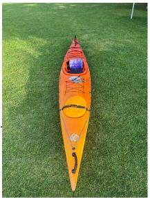
**Details** – Sit-in, good stability makes it suitable for beginners. rudder for easy steering and better control. 22 kg and 3.7m long, two storage hatches
