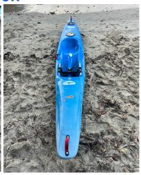
**Details** – the Blue Ski & Green Ski are also known by their model name - Enduro. Designed for maneuverability, speed and stability with an adjustable skeg steering system. Both are sit-on kayaks weighing 17 kgs and 3.8 ms long.
