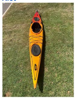
**Details** –designed to balance manoeuvrability and straight line tracking. Sit-in, enclosed cockpit, adjustable pedals controlling a rudder for steering. Two storage hatches, 27 kg and 4.5m long.
