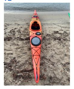
**Details** – T2 Odyssey is a sit-in, sea kayak, heavier than most kayaks in the fleet with adjustable pedals and a skeg. Enclosed cockpit, three storage hatches, made by Wilderness
