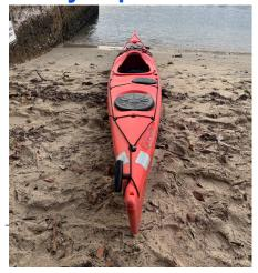
**Details** – made for average size paddlers. It is a heavier kayak with adjustable pedals, skeg, and three storage hatches.
