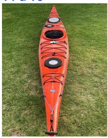
**Details** – sit-in, sea kayak, adjustable pedals and skeg.. Enclosed cockpit with three storage hatches. Manufactured by Wilderness, slightly heavier than other kayaks in the fleet.
