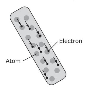
21 Electricity is conducted through some things better than others. Its resistance measures how well something conducts electricity. Some things hold their electrons very tightly. Electrons do not move through them very well. These things are called insulators. Rubber, plastic, cloth, glass and dry air are good insulators and have very high resistance.
