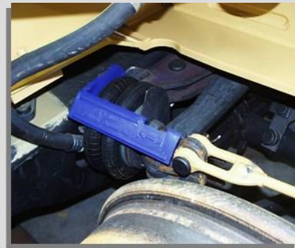
Easily readable indicator area makes inspection faster and safer.
