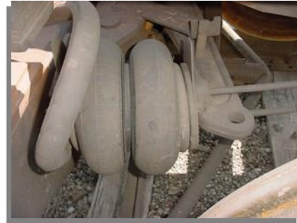
TMB Piston with “Goal Post” Piston Travel Indicator.
