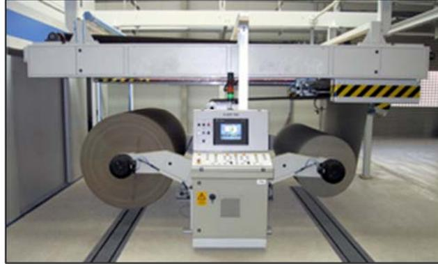
PORTABOBINAS Y EMPALMADOR AUTOMÁTICO DE BOBINAS (SPLICER)
