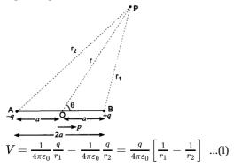
If  $(r, \theta)$  are polar coordinates of point P with respect to mid-point O of dipole, then
