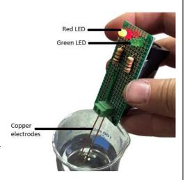
The meter has a 9V battery, two parallel copper electrodes and
