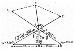
Electric field at the mid point O due to charge at A
