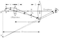
ii. Linear Magnification due to objective lens is given by  $=\frac{\tan \beta}{\tan \alpha}$
