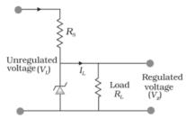
The unregulated dc voltage (filtered output of a rectifier) is connected to the Zener diode through a series resistance  $R_s$  such that the Zener diode is reverse biased.
