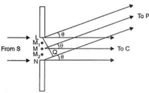
We, therefore, get maxima and minima, i.e., a diffraction pattern, on the screen. **Maxima and minima** are produced when the path difference between waves is a whole number of wavelengths or an odd number of half wavelengths respectively.
