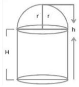
Let the radius of the hemispherical dome be r and the total height of the building be h.
