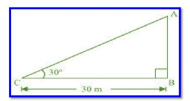
Let AB be the tower and the angle of elevation from point C (on ground) is 30°. In  $\Delta ABC,\,$
