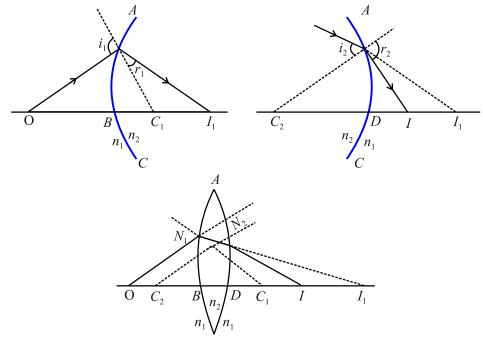
**Step 2:** The image of object O for first surface acts like a virtual object for the second surface. Now for the first surface ABC, ray will move from rarer to denser medium, then
