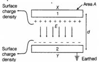
Suppose, the plate X is given a charge of +q coulomb. By induction, -q coulomb of charge is produced on the inner surface of the plate Y and +q coulomb on the outer surface. Since, the plate Y is connected to the earth, hence the relatively weak charge +q residing far away i.e. on the outer surface flows to the earth. Thus, the plates X and Y have equal and opposite charges +q and -q respectively
