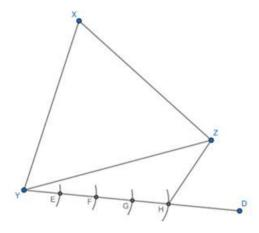
3) Taking H as the center and any radius, draw an arc., intersecting YD and ZH at I and J respectively. Taking G as the center and radius HI, draw an arc., intersecting YD at K. Taking K as the center and radius IJ, draw an arc, intersecting previous arc at L. Join and extend HL, intersecting YZ at M.
