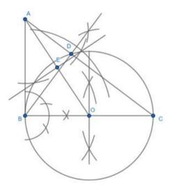
Step 6: We construct the perpendicular bisector of AO, which intersects it at point E.
