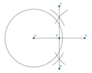
Step 3: Construct perpendicular bisector AB of line segment OP. Point E is where they intersect.
