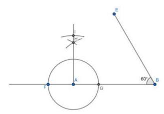
3) Keeping I as the center, draw a circle of any radius, intersecting extended AH at J and K. Keeping J as the center and any radius draw a circular arc. Now, Keeping K as the center and same radius as before, draw another arc, intersecting previous arc at L. Join and extend IL, intersecting BE at C. Join AC.
