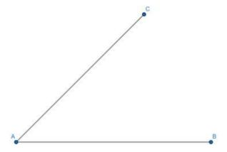
Step 1: Draw a line segment AC of arbitrary length and at an any angle to AB such that ∠CAB is acute.
