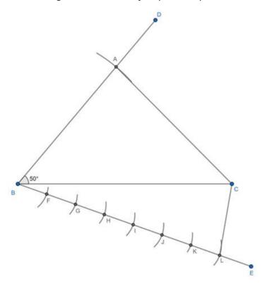
4) Taking L as the center and any radius, draw an arc., intersecting BE and CL at M and N respectively. Taking J as the center and radius LM, draw an arc., intersecting BE at O. Taking O as the center and radius MN, draw an arc, intersecting previous arc at P. Join and extend JP, intersecting BC at Q.
