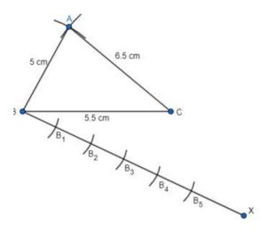
Step 4.  $B_3$  is joined with C to form  $B_3$  C as 3 point is smaller.  $B_5$   $C_1$  is drawn parallel to  $B_3$  C as 5 point is greater.
