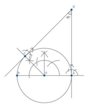
$\underline{\text{Step 4}}$ : We extend the perpendiculars to meet at point D, and we get tangents AD and CD to the circle, enclosing 45° between them.
