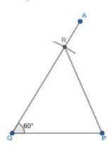
3) Draw any line segment QB, making an acute angle with PQ and opposite to the vertex R. Taking Q as the center and any radius, draw an arc, intersecting QB at C. Taking C as the center and radius QC, draw an arc, intersecting QB at D. Similarly, repeat the process 3 more times to get points E, F and G. Join PG.
