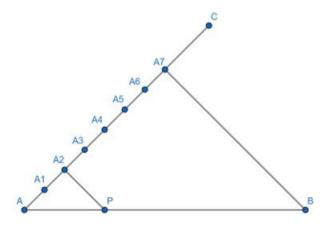
Step 4: We draw line segment  $A_2P$  such that  $A_2P \parallel A_7B$  and P is the point of intersection of this line segment with AB.
