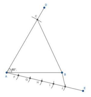
4) Taking J as the center and any radius, draw an arc., intersecting AE and BJ at K and L respectively. Taking I as the center and radius JK, draw an arc., intersecting AE at M. Taking M as the center and radius KL, draw an arc, intersecting previous arc at N. Join and extend IN, intersecting AB at O.
