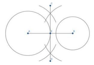
Step 3: We construct perpendicular bisector CD of line segment AB. They intersect at point E.
