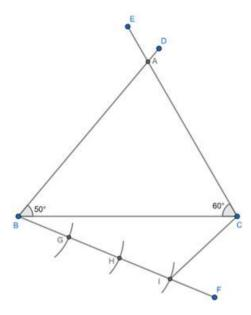
4) Taking I as the center and any radius, draw an arc., intersecting BF and CI at J and K respectively. Taking H as the center and radius IJ, draw an arc., intersecting BF at L. Taking L as the center and radius JK, draw an arc, intersecting previous arc at M. Join and extend HM, intersecting BC at N.
