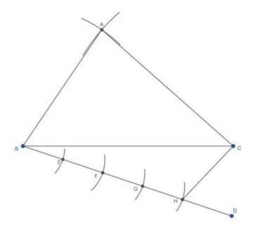
4) Taking H as the center and any radius, draw an arc., intersecting BD and CH at I and J respectively. Taking G as the center and radius HI, draw an arc., intersecting BD at K. Taking K as the center and radius IJ, draw an arc, intersecting previous arc at L. Join and extend HL, intersecting BC at M.
