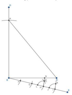
5) Taking C as the center and any radius, draw an arc., intersecting BC and CA at P and Q respectively. Taking N as the center and radius CP, draw an arc., intersecting BC at R. Taking R as the center and radius PQ, draw an arc, intersecting previous arc at S. Join and extend NS, intersecting AB at O.
