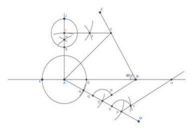
6) Taking B as the center and any radius, draw an arc., intersecting BA and BC at W and X respectively. Taking U as the center and radius BW, draw an arc., intersecting AU at Y. Taking Y as the center and radius WX, draw an arc, intersecting previous arc at Z. Join and extend UZ, intersecting extended AC at V.
