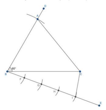
4)Taking I as the center and any radius, draw an arc., intersecting BD and CI at J and K respectively. Taking H as the center and radius IJ, draw an arc., intersecting BD at L. Taking L as the center and radius JK, draw an arc, intersecting previous arc at M. Join and extend HM, intersecting BC at N.
