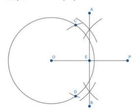
Step 4: Taking OE as the radius and centre at E, we draw arcs to cut the circle at points C and D.
