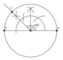
Step 2: We construct an angle of 135° at centre O, such that  $\angle AOC = 135^{\circ}$ , where C is another point on the circle.
