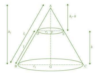
Let ABC be a cone. A frustum DECB is cut by a plane parallel to its base. Let  $r_1$  and  $r_2$  be the radii of the ends of the frustum of the cone and h be the height of the frustum of the cone.
