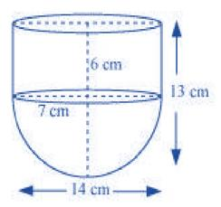
It can be observed that radius (r) of the cylindrical part and the hemispherical part is the same (i.e., 7 cm).
