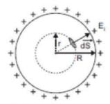
The charge resides on the surface of a conductor. Thus, a hollow charged conductor is equivalent to a charged spherical shell. Let's consider a spherical Gaussian surface of radius (r < R). If E is the electric field inside the shell, then by symmetry electric field strength has the same magnitude  $E_i$  on the Gaussian surface and is directed radially outward.
