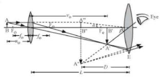
where AB = object, A'B' = image formed by objective, A"B" = image formed by eyepiece
