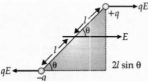
Consider electric dipole kept in a uniform electric field. Consider electric dipole kept in a uniform electric field at an angle  $\theta$  where a dipole experience a torque, so, the torque generated by parallel forces qE will act as a couple as
