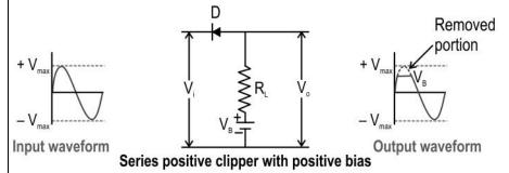
During the positive input half cycle, the diode is reverse biased by the input supply voltage  $V_i$ . But since the positive terminal of the battery is connected to p-side and the negative terminal of the battery is connected to n-side of the diode, the diode is forward biased by the battery voltage  $V_B$ .
