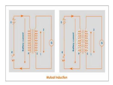
Similarly, when the key is released, magnetic flux associated with the coils decreases and this gives rise to induced current in the direction shown by the arrow marked 2.
