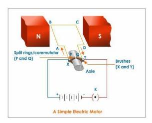
When the coil turns through  $90^{\circ}$ , the brushes lose contact with the commutator and the current stops flowing through the coil.
