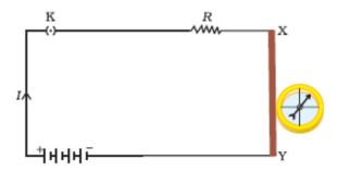
The needle is deflected which means that the electric current through the copper wire has produced a magnetic effect.
