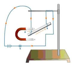
A current carrying conductor experiences a force when placed in a magnetic field. The direction of force is reversed when the direction of current in the conductor is reversed.
