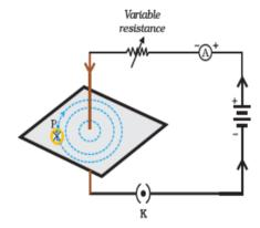
If the current in the copper wire is changed, the deflection in the needle also changes. In fact, if the current is increased, the deflection also increases.
