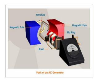
Armature is a soft iron core on which a coil having a large number of turns of insulated copper wire is wound. Magnetic poles are concave and cylindrical. The concave poles produce a radial magnetic field.
