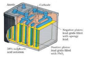
When the battery is in use, the following cell reactions take place:
