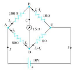
A galvanometer of  $15\Omega$  resistance is connected across BD. Calculate the current through the galvanometer when a potential difference of 10~V is maintained across AC.
