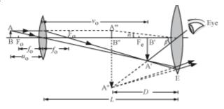
where AB = object, A'B' = image formed by objective, A"B" = image formed by eyepiece
