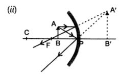
Nature of image: Virtual, enlarged and erect image is formed behind the mirror.
