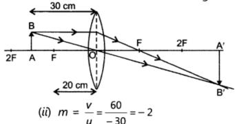
So, image is inverted and double the size of the object.
