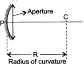
(ii) The radius of the sphere of which the reflecting surface of the spherical mirror forms a part is called the radius of curvature of the mirror.
