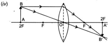
Nature of image: Real, inverted and size to size, image is formed at 2F on the other side of lens.
