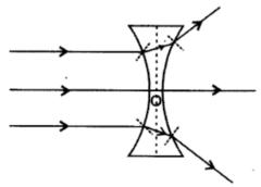
Thus, because of the concave shape of both the faces, the double concave lens diverge the rays of parallel beam of
