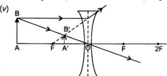
Nature of image: Virtual, erect and diminished image is formed between O and F on the same side of object.
