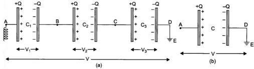
In series first plate of each capacitor has charge +Q and second plate of each capacitor has charge -Q i.e., charge on each capacitor is Q.
