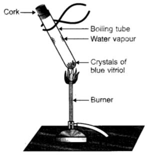
Materials Required: CuS04.5H20 (Blue vitriol), boiling tube, burner, cork, delivery tube, test tube, clamp stand.
