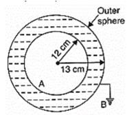
$$\begin{split} C &= kC_0 \\ C &= k.4\pi\varepsilon_0 \frac{r_1 r_2}{r_2 - r_1} \\ &= \frac{32 \times 13 \times 10^{-2} \times 12 \times 10^{-2}}{9 \times 10^9 (13 \times 10^{-2} - 12 \times 10^{-2})} \Big[ \because 4\pi\varepsilon_0 = \frac{1}{9 \times 10^9} \Big] \\ &= \frac{32 \times 13 \times 12}{9} \times 10^{-11} = \frac{1644}{3} \times 10^{-11} \\ &= 5.54 \times 10^{-9} F \end{split}$$
