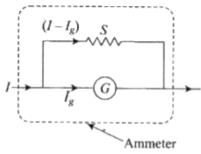
For measuring  $I_1 = 10 \text{ mA} : I_g.G = (I_1-I_G)(S_1 + S_2 + S_3)$
