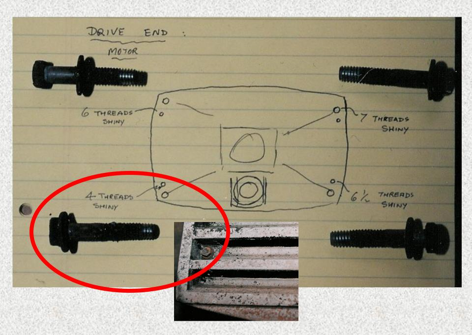
88 О О 6 THREADS 7 THREADS ø SHINY SHINY 1.0"(LESS WASHER) D. 85 FROM FACE TO BELOW FROM FACE WASHER ٥-P 6 THREADS 4 THREADS SHINY 0.9" FROM PACE 0.9 FROM FACE TO BELOW WASHER · 16 THREADS/ INCH · \$ 5/16" BOLTS X 1 4 "LG. 1.221 SHROUP TO (ASTING · WASHERS: D.075 THICK LOOSE FIT THREADS IMPACT MARKS AROUND PERIMETER OF SHROUD. METALLIC RATTLING IF BOLTS LOOSE SHROUD (VIEW FROM BOTTOM) NO GAP 0.004" 0.058 0.045" MOTOR BRACKET ·012 © HALES & GOOCH LTD.
