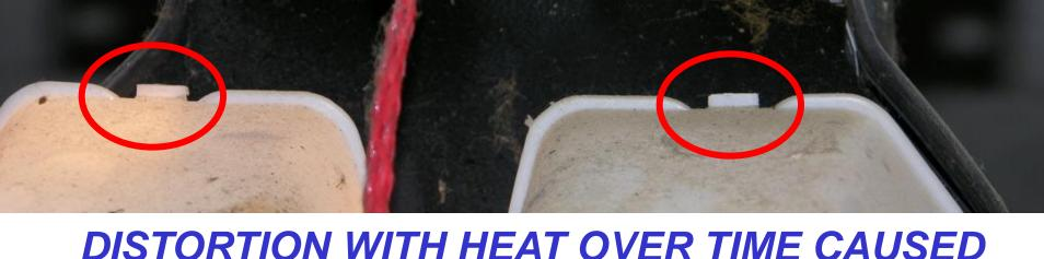
DISTORTION WITH HEAT OVER TIME CAUSED
