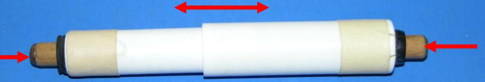
Radially offset axial reaction forces on original plastic stubs cause diaphragming of ends and overload failure.
