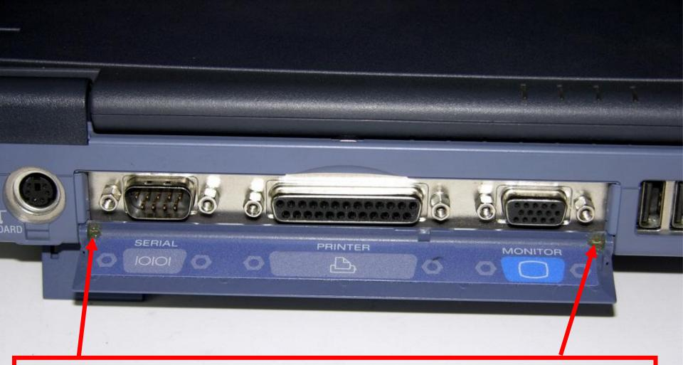
Tiny plastic hinge nibs broke off and door fell out
