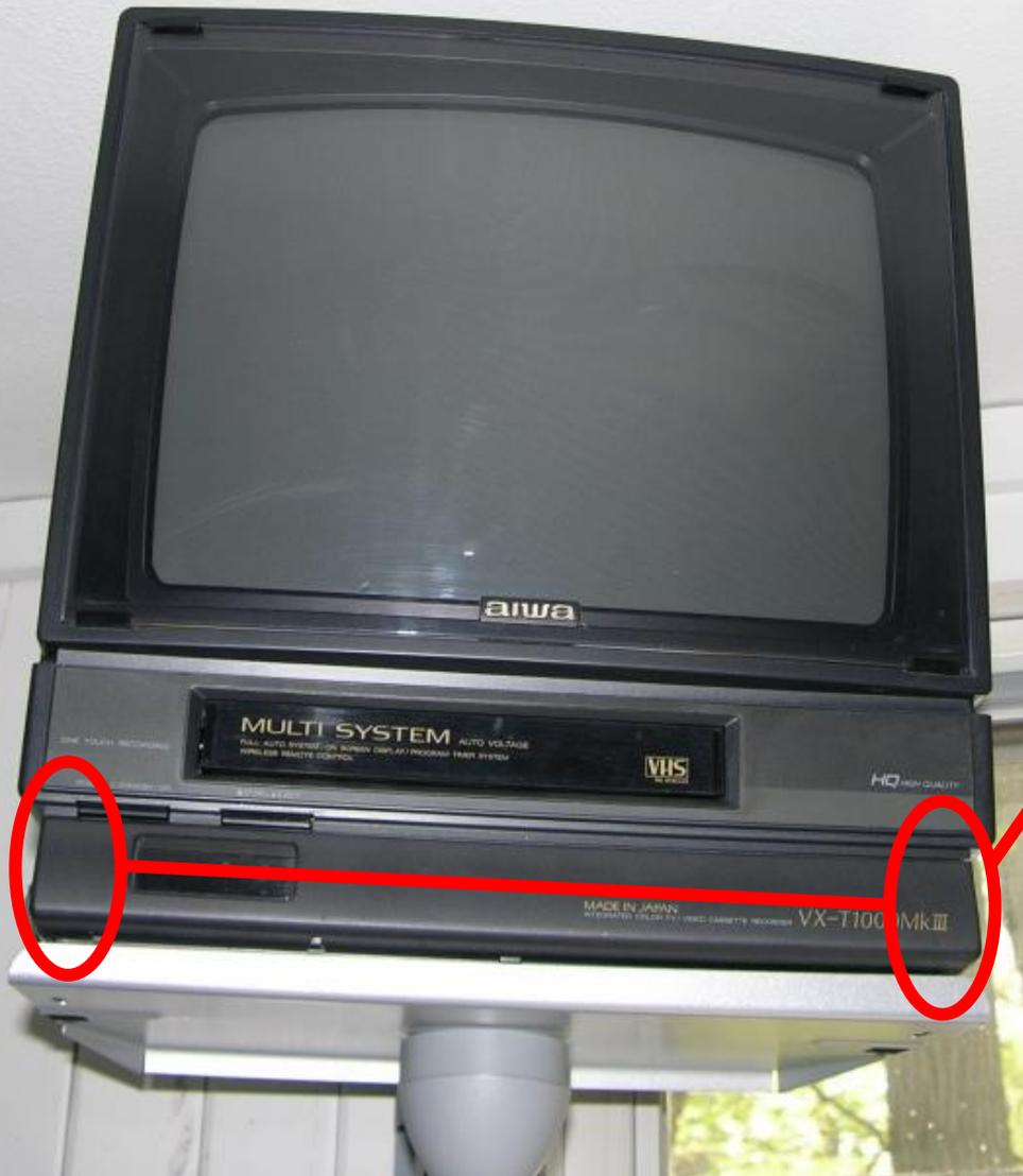
*Plastic spring clips relaxed to point of failure to hold.*
