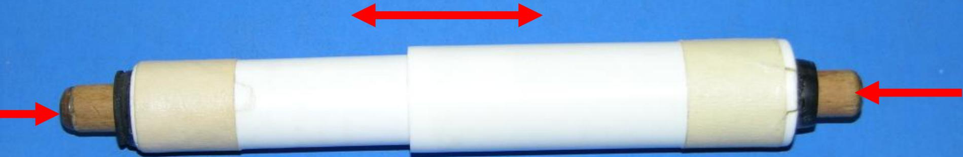
**Radially offset** axial reaction forces on original plastic stubs cause diaphragming of ends and overload failure.
