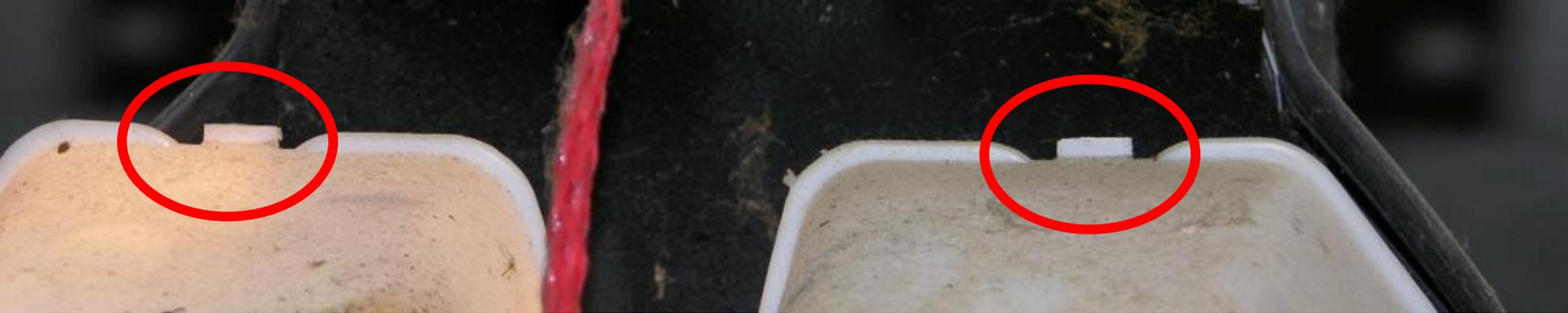
***DISTORTION WITH HEAT OVER TIME CAUSED
