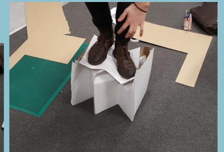
FAILED Components not strong enough. try double wall.
