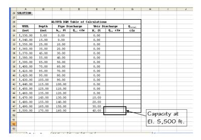
ii) Now adjust the Spillway Coefficient, C<sub>w</sub>, in the "Given" section until the calculated Weir Discharge, Q<sub>w</sub>, is within ±10 cfs of the value you found in the previous step. Keep adjusting the C<sub>w</sub> value manually to 3 decimal places.
