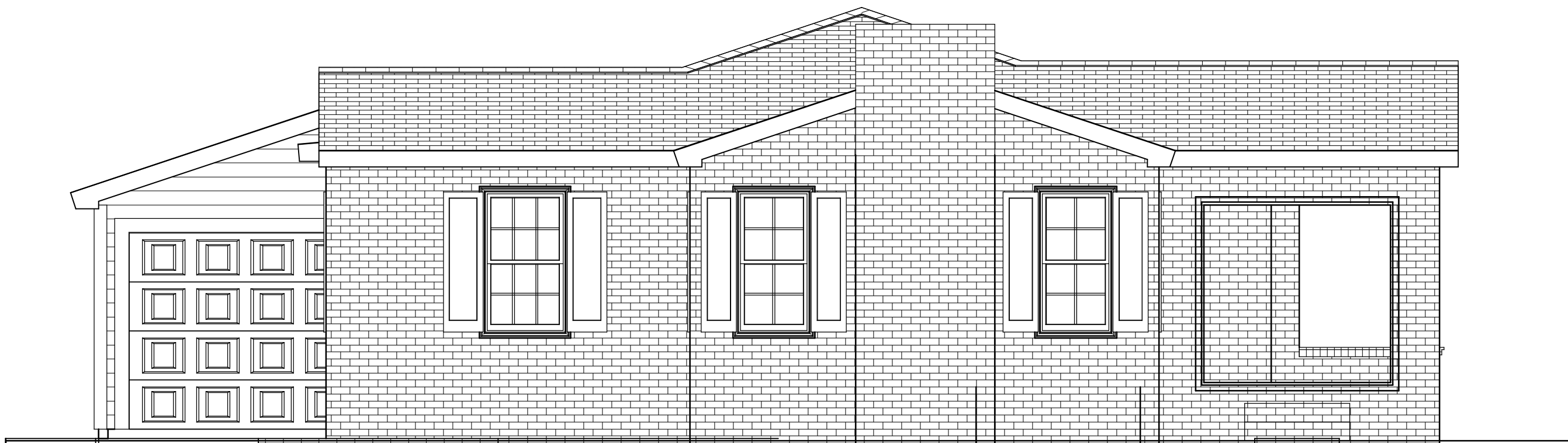
FRONT AS-BUILT ELEVATION
