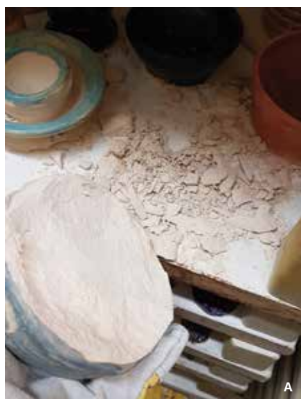
A The aftermath of a clay explosion in a bisque firing due to firing wet pots. B Check for moisture during candling. When my safety glasses fog up it means there is still moisture escaping and candling the kiln should continue.
