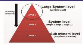
> To determine design parameters of carrier vehicle (Level 0), a top down approach is developed and intelligent solution is evovled
