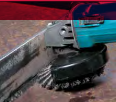
Cleaning a corner weld with a bevel brush.
