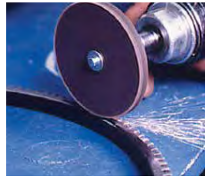
A unitized wheel deburring a ring gear.
