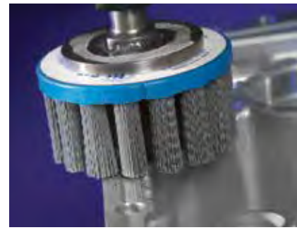
Deburring the edges of an aluminum engine cover.
