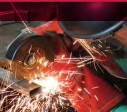
UltraCut wheel making precision cuts on steel tube stock.
