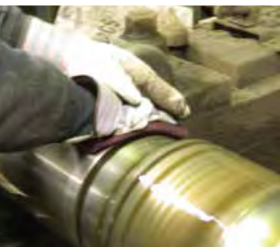
Polishing a rail axle journal with a non-woven hand pad.
