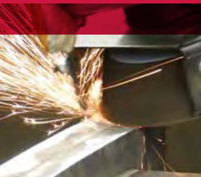
Type 11 Cup Rock for snagging and heavy stock removal.
