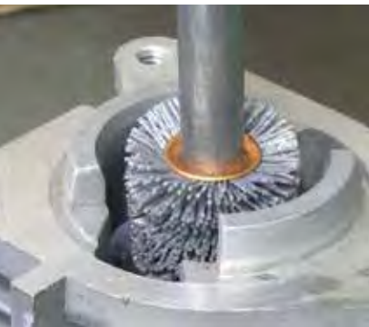
Deburring internal bores of a cylinder head.
