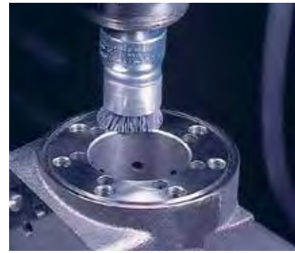
Blending tool marks on a hydraulic component.
