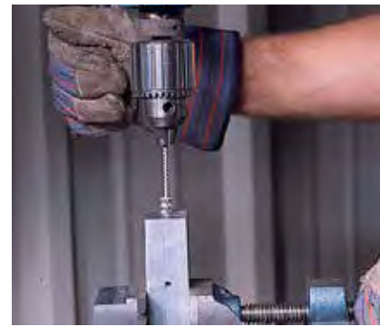
Crosshole deburring an aluminum manifold.
