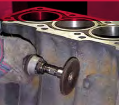
Removing flash from a sand-cast iron engine block.
