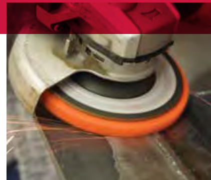
Weld cleaning with a strip disc.
