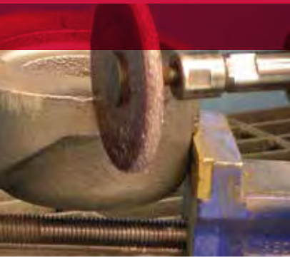
Removing casting flash from ductile-iron housing with an encapsulated brush.
