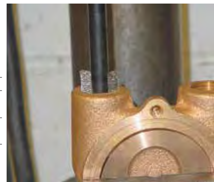
Deburring the threads of a tapped hole using a burrite brush in a holder.
