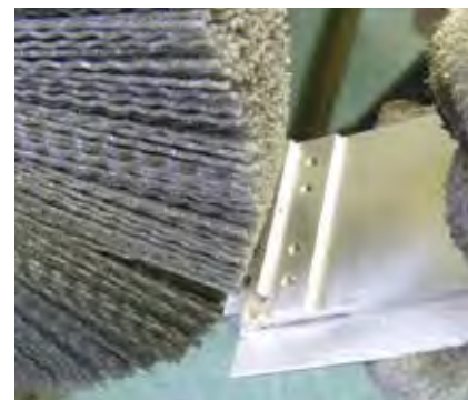
Removing burrs from an aluminum heat sink.
