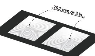
Carefully cut the transparent tape and reposition the optical center. A simple shift in or out a few mm will be enough to accomodate your interocular distance.
